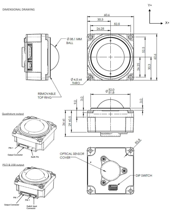
Dimensional drawing specifies factory default orientation. All dimensions are in mm unless otherwise stated.
