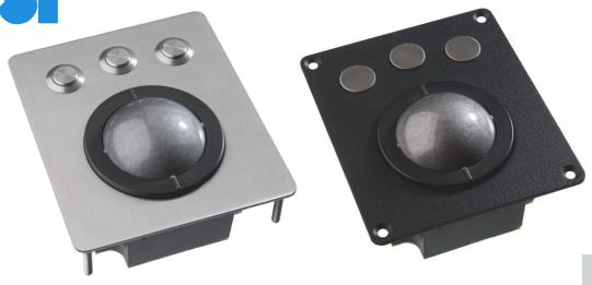
• 50 mm ball • IP65/IP68 sealing stainless steel carrier
