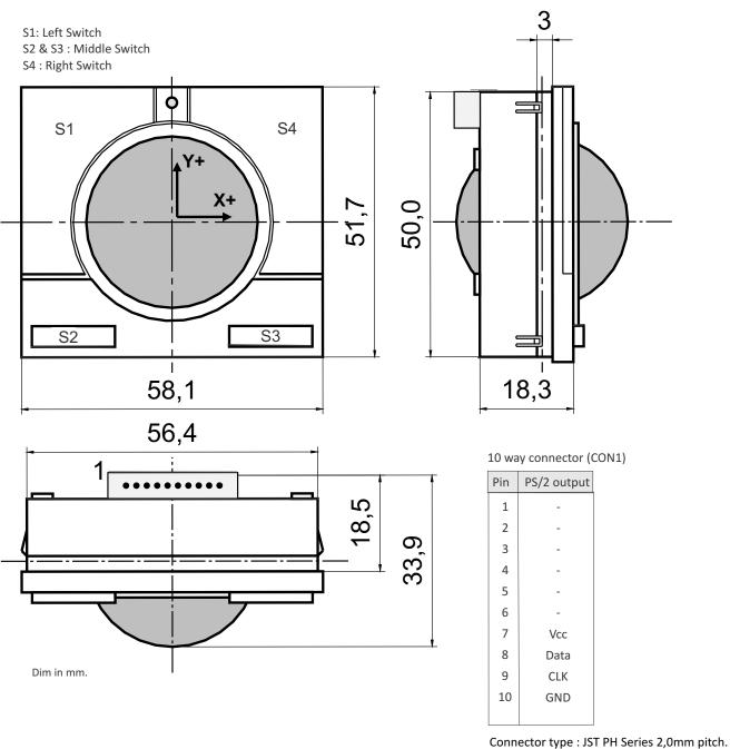
Connector type : JST PH Series 2,0mm pitch. Mating part : JST KR Connectors (10KR-8M)
