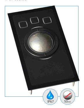
The TBX50B1 trackball is a ruggedized trackball, specially designed for harsh industrial environment applications: the self-adjusting PTFE seal of the trackerball guarantees an IP67 protection grade. This laser trackball has a large 50 mm diameter ball, which make this unit the ideal solution for all applications where accurate pointer control is required.
