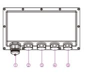
1. 1 x IP67 USB 2.0 A Type with cover 2. 1 x IP67 LAN with RJ45 Connector 3. 1 x IP67 USB 2.0 Connector 4. 1 x IP67 RS232/422/485
