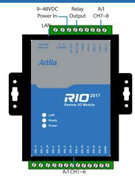
RIO-2017 is an analog input remote I/O module supports Bluemix IoT and Web API. The analog input channel can be configured as current and voltage and it is auto calibrated and 2500Vrms isolated. In addition to the analog input, RIO-2017 also has one relay output. Therefore it is suitable for remote data acquisition and control. RIO-2017 supports web RESTful interface for web based application to access its analog and digital I/O.
