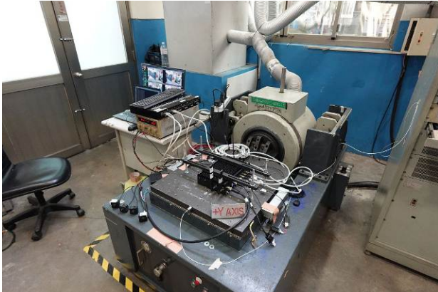
FIG 11.1: +Y axis direction mounted
