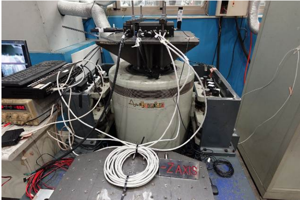
FIG 17.1: -Z axis direction mounted
