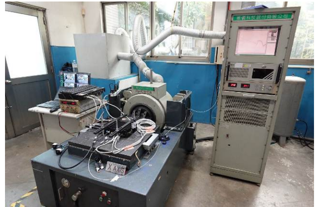
FIG 1.2: X axis direction mounted
