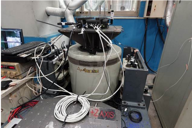
FIG 15.1: +Z axis direction mounted
