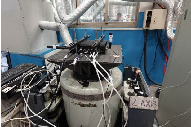
FIG 5.1: Z axis direction mounted
