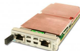
AMC720 Xeon E3-1125 Processor AMC
