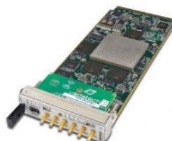
AMC526 MC Dual ADC, Virtex-7, 12-Bit @ 2.6 GSPS
