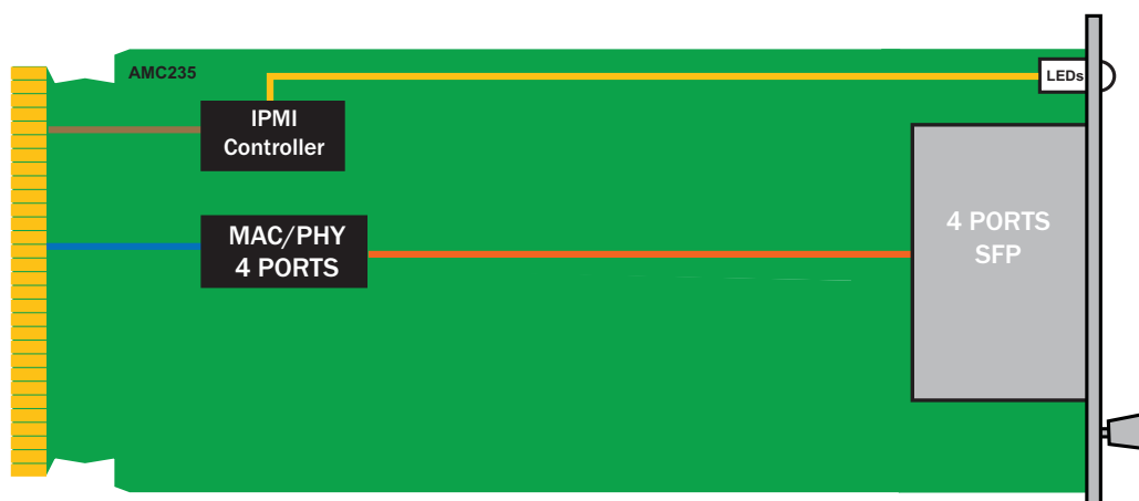
FIGURE 1. AMC235 Functional Block Diagram
